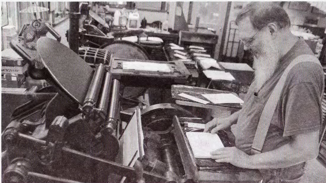
Larkspur Press founder, master printer and guru Gray Zeitz feeds each page through the hefty Chandler & Price letterpress.
